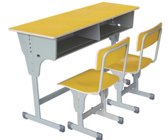
5206 double-seat adjustable height desk & chair Desk & chair panel : 1.6(1.0)cm plywood hot-press fireproof board,trimming paint Desk & chair frame: 20x49x1.0mm oval tube Desk drawer: side board 1.0mm drawer board 0.7mm
